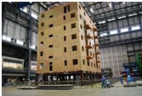
Figure 1 : Dynamic testing of a real-scale building
