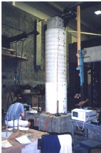
Figure 1 : Reinforced concrete column tested up to failure
