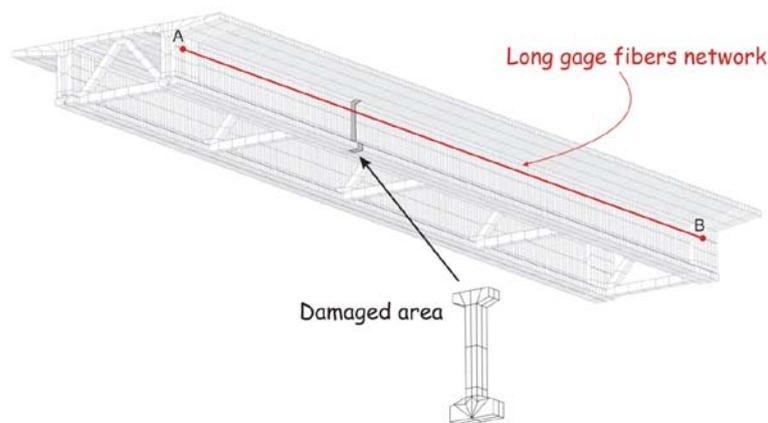
Figure 1 : Finite element model of a concrete bridge with simulated damage and dynamic strain sensors attached to it for damage localization
