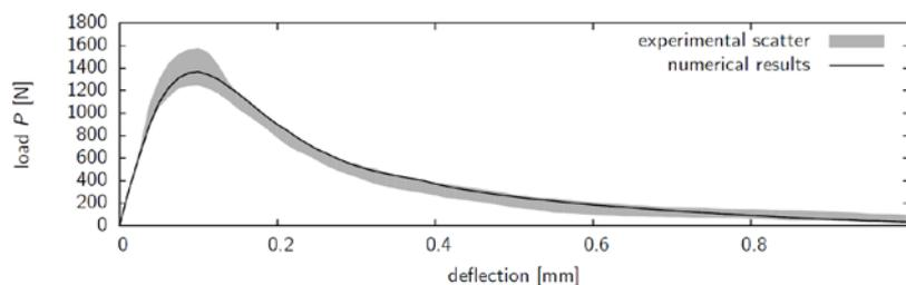
Figure 2: Experimental and numerical load-deflection-curve
