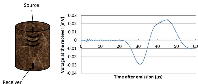
Figure 1 : Soil sample and transmitted ultrasonic wave
